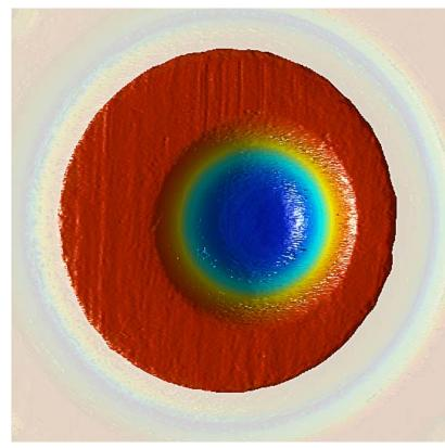
Automatic segmentation of the primer cup by exploiting normal vectors
